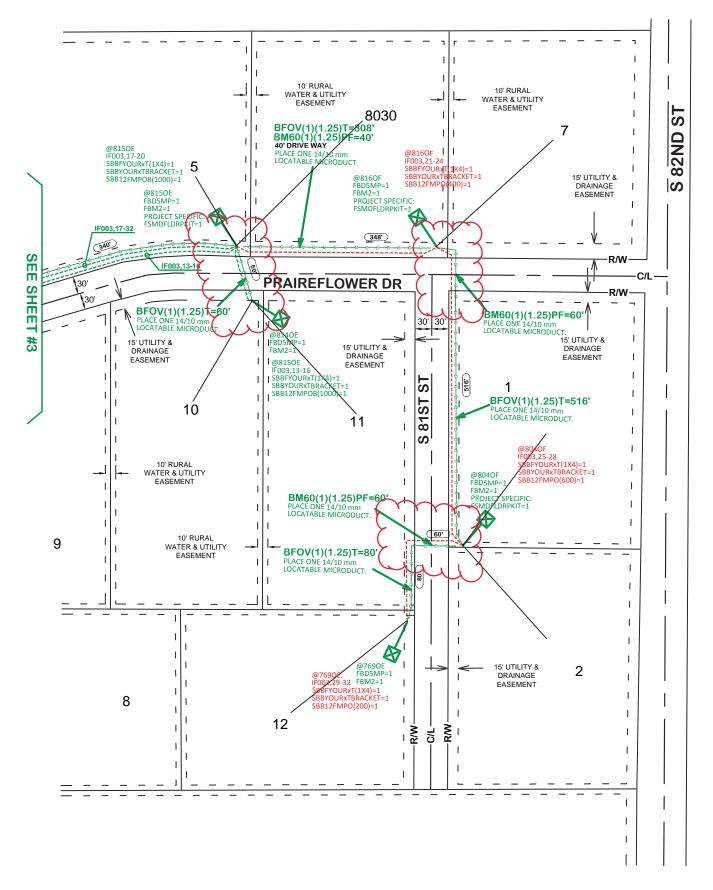
All Road Crossings Must Be A MINIMUM Of 48" Below The Flow Line Of The Ditch.
