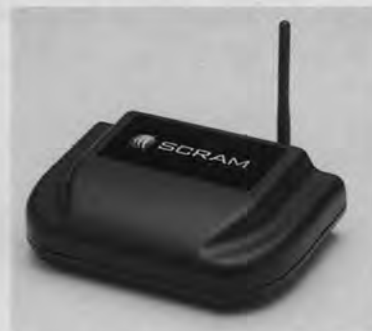
The optional cellular-based radio frequency (RF) base station provides a more granular layer of supervision and enhances the battery life in the tracking device when the client enters the area where the base station is located. The system automatically switches from GPS tracking to traditional RF/house-arrest monitoring.
