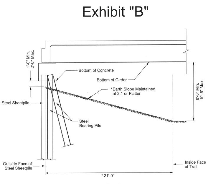
\* Measured Perpendicular to Centerline of Support Note: Not to Scale
