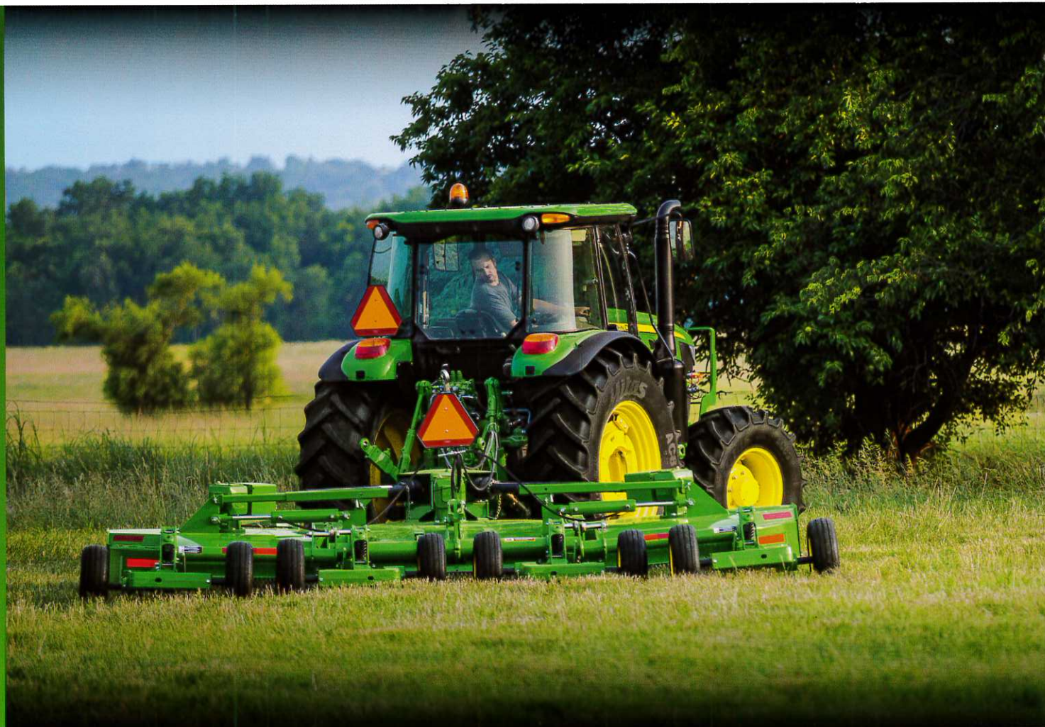
Take on a wide range of PTO-powered jobs with the 540/1000 RPM independent PTO system.
