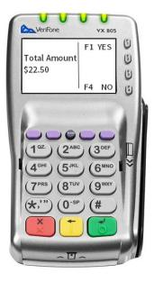
The VX 805 is the external pin entry device (aka pin pad). It is plugged directly into the VX 520 through an RS232 connector cable, which is supplied by LexisNexis. The purpose of the VX 805 is to allow secure data entry for a debit card PIN number.
